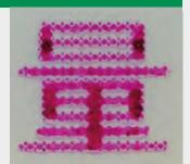
In confronto, un'incisione standard con HelioKlischograph / In comparison, a standard engraving with HelioKlischograph
